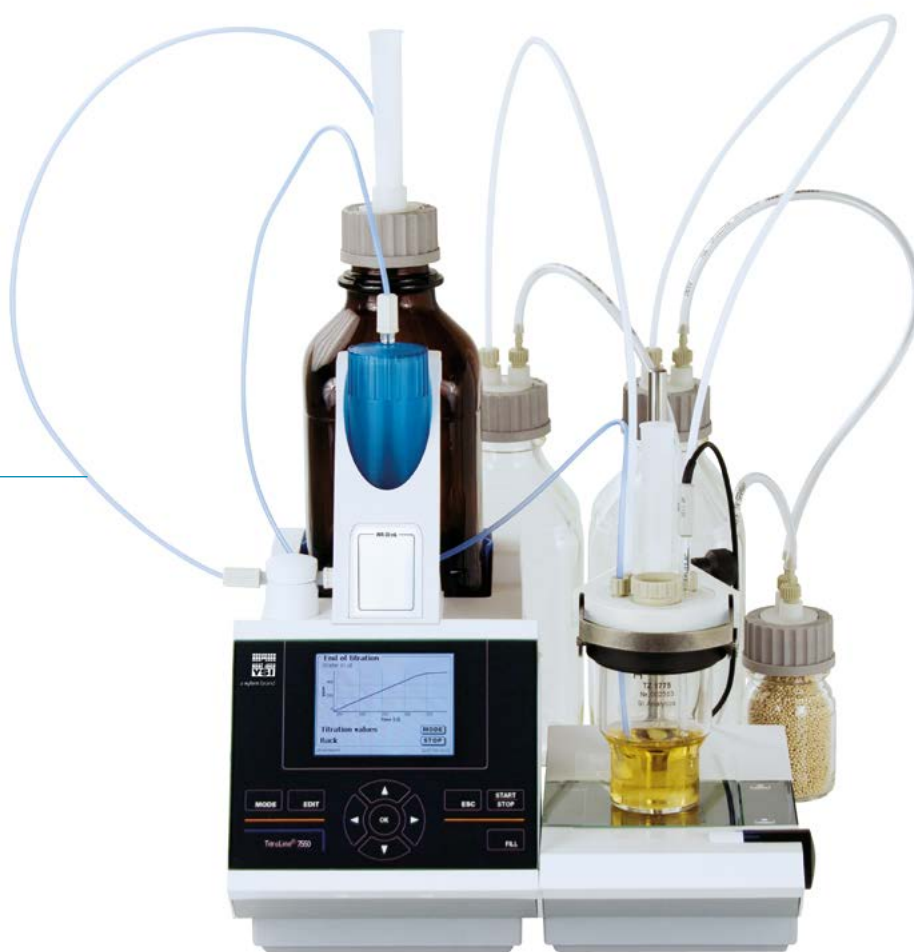
TitroLine® 7750 with accessories for KF titration
